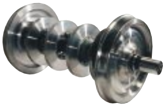
TGV trailer wheelset equipped with four brake discs.
