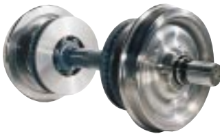
Wheelset for the Eurotunnel shuttle.
