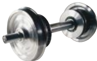
Wheelset designed for speeds up to 160 km/hour.
