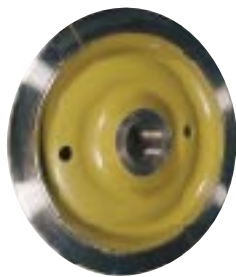
Wheel with noise-damping ring.
