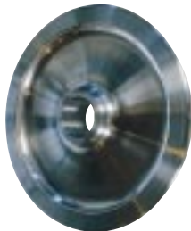
Standard wheel for urban traffic (with noise damping system)
