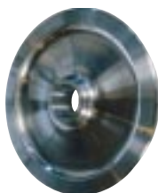
Locomotive wheel with noise damping ring.
