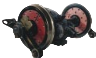
Power wheelset with final drive unit and brake discs bolted onto the wheels.
