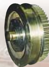
Crane wheel and shaft fitted with a drive unit
