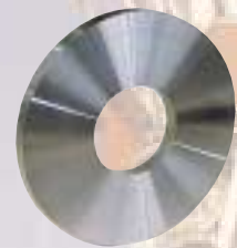
High-performance brake disc for high speed trains
